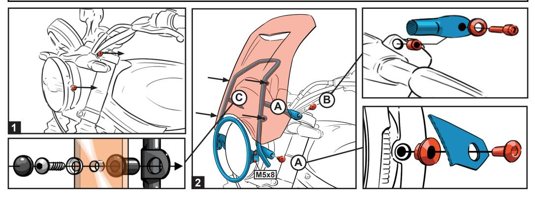
**EN** It is important to tighten the screws only after all parts have been assembled. Start by inserting the screws without tightening them.
