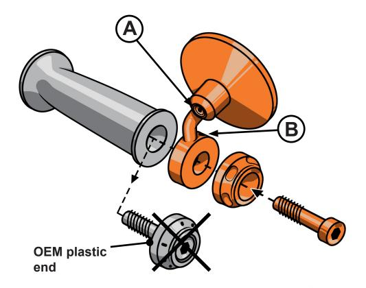
EN\_If made out of plastic, remove the OEM end and mount the Unit Garage's mirror and end as shown in the scheme. For a correct and safe mounting: tighten the screws with the mirror in position, go for a test ride and then tighten again the screws.
