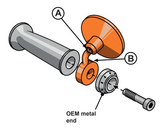
EN\_Remove the OEM end, mount the mirror and put everything back on as shown in the scheme. For a correct and safe mounting: tighten the screws with the mirror in position, go for a test ride and then tighten again the screws.
