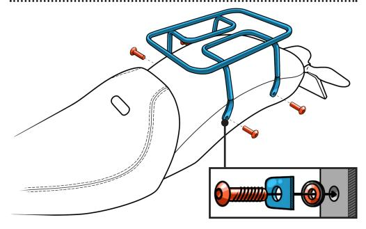
**EN** Remove the screws from both sides of the rear mudguard.
