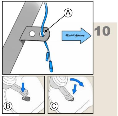
8 Mount the windscreen with support onto the subframe as shown in the image. In (8A) fit the M8x16 screw, use the metal washer and locknut on the inside. In the adjustable slot (8B) fit the M8x16 and included black plastic washer underneath the screw head. In (8C) fit the M8x25 screw to mount the headlight housing, using the 2 black aluminium spacers on either side of the headlight housing.
